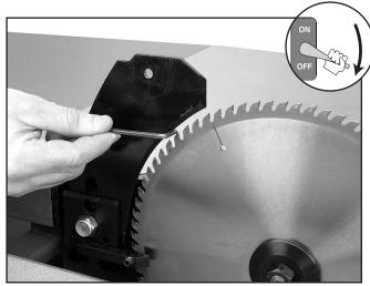
Figure 32. Adjusting the riving knife.
